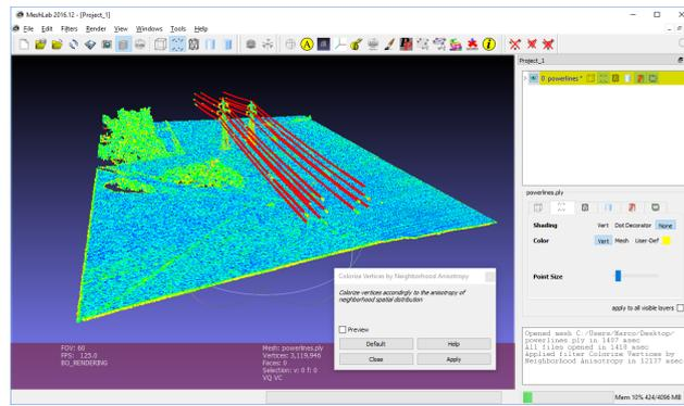
Fig. 1.2: Powerline 3D points classification, MeshLab experimental plug-in.
