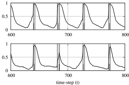
Figure 5: Excitatory strategy: neural activation and signalling status for two of the ten robots. The bold line indicates the activation of the neuron  $N_{O,3}$ , which controls the flashing signal. The vertical grey bands indicate the perceived signal  $s(t)$ . The small dark vertical lines within the grey band indicate the time-step in which the robot itself is signalling. The plot refers to a density  $d = 0.2$ .
