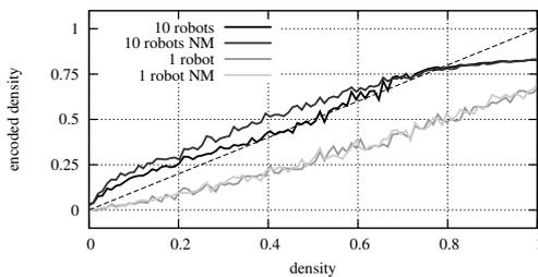
Figure 11: Encoded density for varying group size and for blocked. Each line represents the average of 100 trials, performed for 100 density values in  $[0, 1]$ . Data for 1, 2, 3, 4 and 10 robots are shown.
