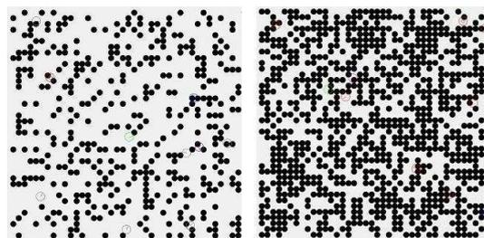
Figure 1: Two snapshots of the simulated arena are shown. The black disks spots are painted on a grey floor. The spots are positioned on a grid of  $40 \times 40$  cells. The density (i.e. the probability to find a spot in a cell) varies in the range  $[0, 1]$  (left:  $d = 0.26$ , right:  $d = 0.66$ ).
