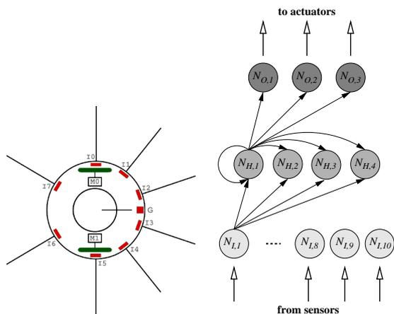
Figure 2: The robot and the neural controller. Left: a schema of the simulated robot. Eight proximity sensors ( $IR_{0-7}$ ) are positioned at  $3.25\text{cm}$  from the ground pointing horizontally. The sensors detect obstacles at a maximum distance of  $\approx 5\text{cm}$ . The floor colour is perceived through an infrared sensor ( $G$ ) positioned on the robots’ front and pointing the floor. Right: the agents’ controller is a CTRNN with 10 sensory neurons, 4 hidden and three motor units.
