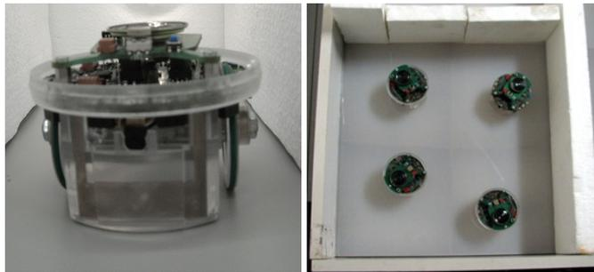
**Fig. 1.** Left: E-puck robot. Right: a group of four epuck robots inside a box shaped arena of 40x40cm
