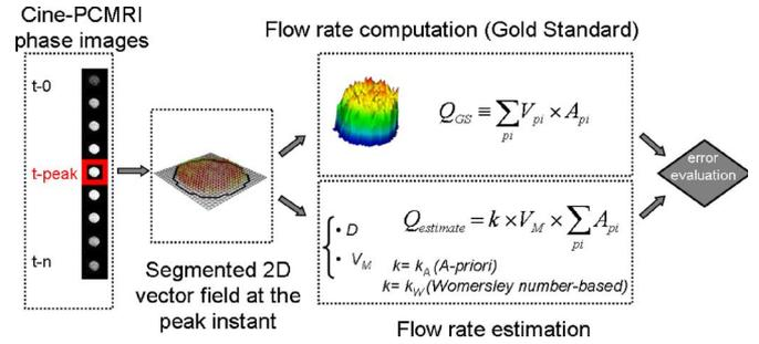
Fig. 2. *In vivo* protocol scheme. At the peak velocity instant the PCMRI dataset has been used in two ways. (Top) PCMRI blood flow-rate computation ( $Q_{GS}$  gold standard). (Bottom) Flow-rate estimates using the *a priori* ( $Q_A$ ) and the Womersley number-based ( $Q_W$ ) approaches.
