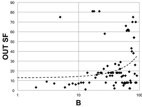
Fig. 5: How the structural features in the target metamodel influence the number of bindings
