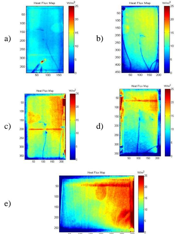
Figure 3: Heat flux map of each roll container surface (in respect to the air stream direction): a) front surface, b) back surface, c) right surface, d) left surface, e) top surface.
