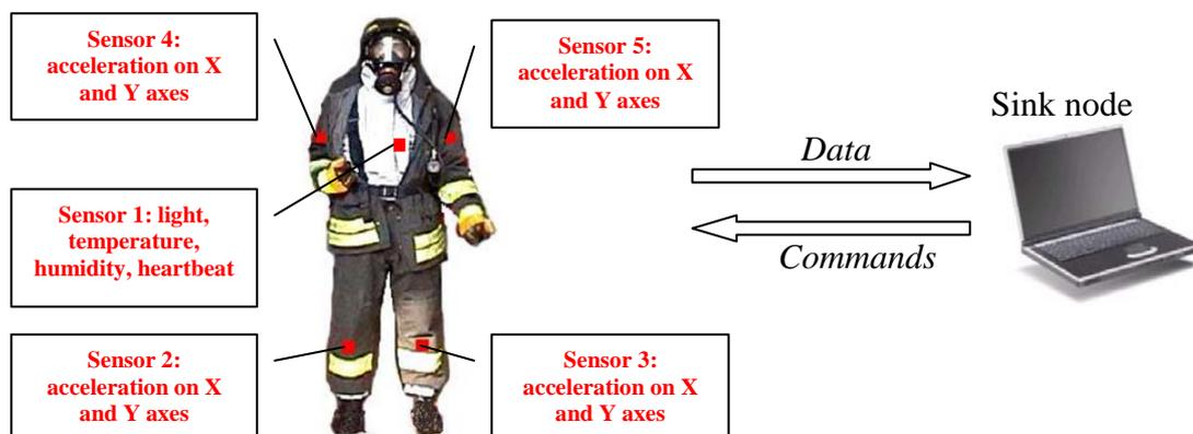
Figure 2. The body area wireless sensor network model.
