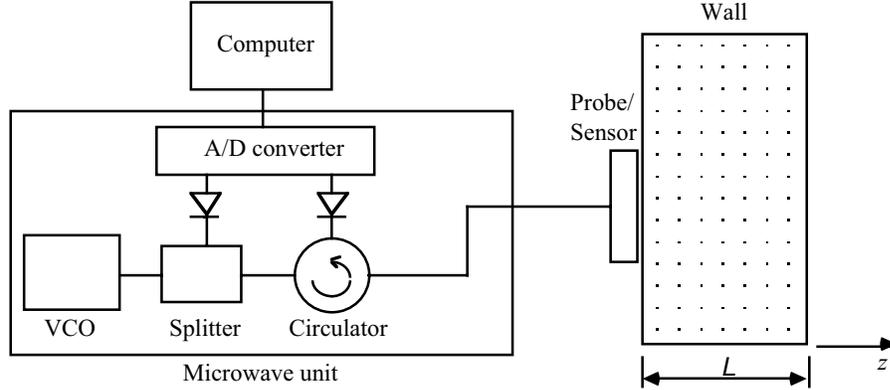
**Fig. 1:** *Monostatic measurement setup*
