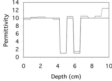
**Fig. 3:** Simulated concrete wall with relative permittivity 10, with two air inclusions 0.833 cm apart. Number of layers assumed: 12. Simulated noisy data with 25 dB SNR. Solid line: original permittivity profile. Dotted line: reconstructed profile.
