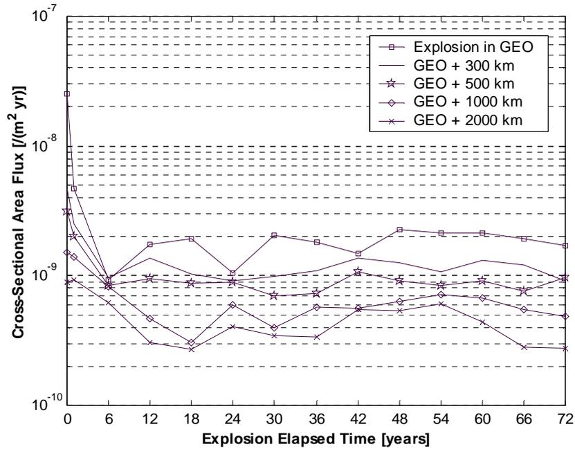
Figure 13. Flux of explosion fragments  $\geq 1$  mm in geostationary orbit, as a function of the breakup altitude and elapsed time
