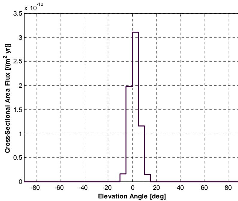
Figure 8. Flux of debris  $\geq 10$  cm in geostationary orbit, as a function of elevation, due to an explosion in GEO (explosion elapsed time = 24 years)
