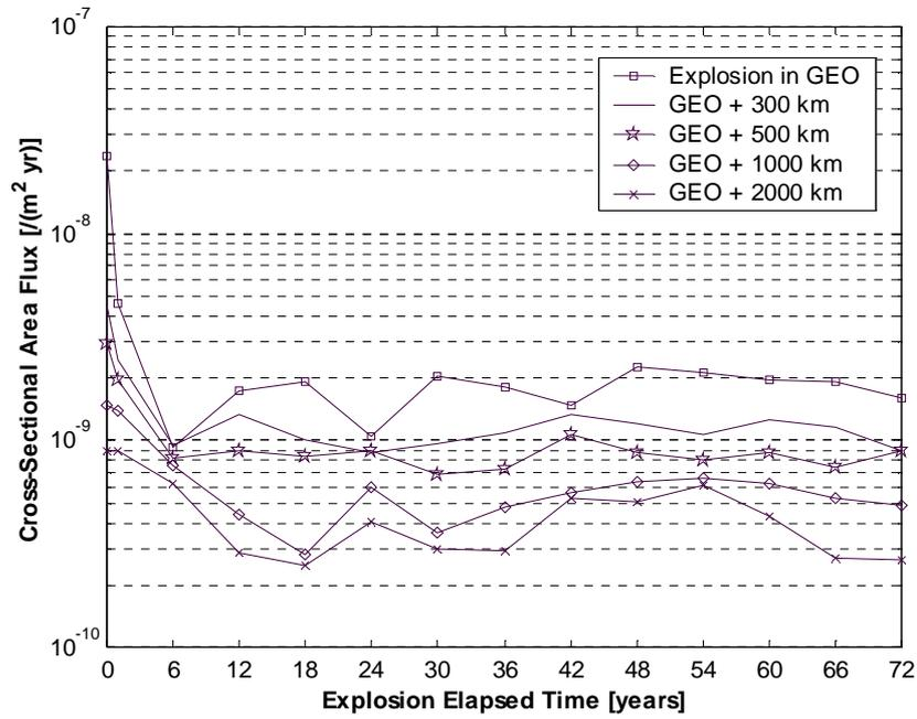
Figure 14. Flux of explosion fragments  $\geq 1$  cm in geostationary orbit, as a function of the breakup altitude and elapsed time
