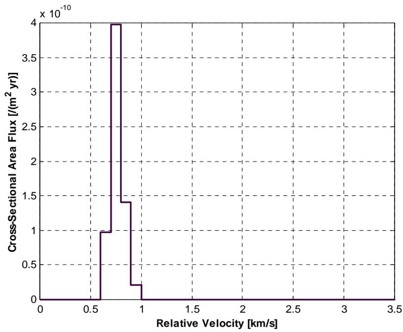
Figure 9. Flux of debris  $\geq 10$  cm in geostationary orbit, as a function of relative velocity, due to an explosion in GEO (explosion elapsed time = 24 years)
