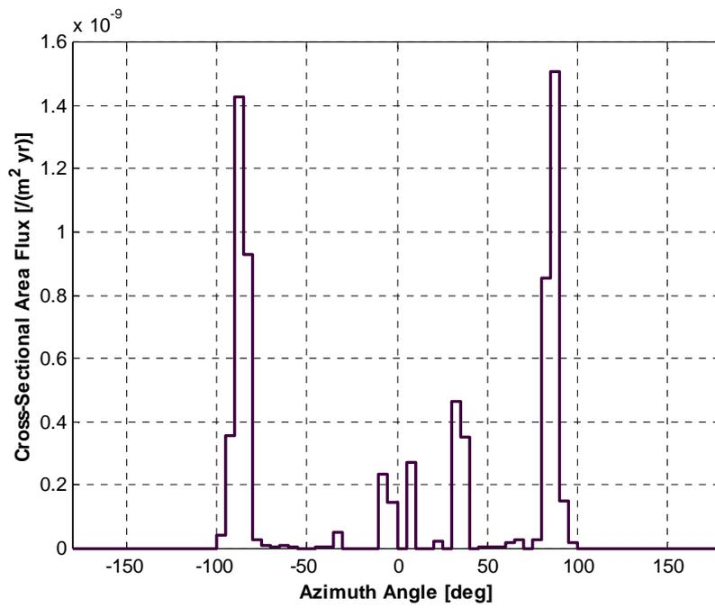
Figure 1. Background flux in GEO, as a function of azimuth, of debris  $\geq 10$  cm
