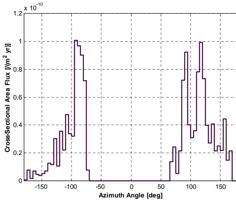
Figure 10. Flux of debris  $\geq 10$  cm in geostationary orbit, as a function of azimuth, due to an explosion in GEO (explosion elapsed time = 54 years)
