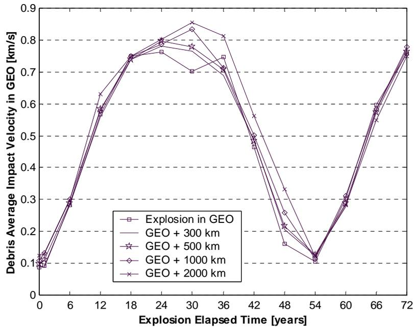
Figure 16. Time evolution of the debris average impact velocity in geostationary orbit as a function of the explosion altitude
