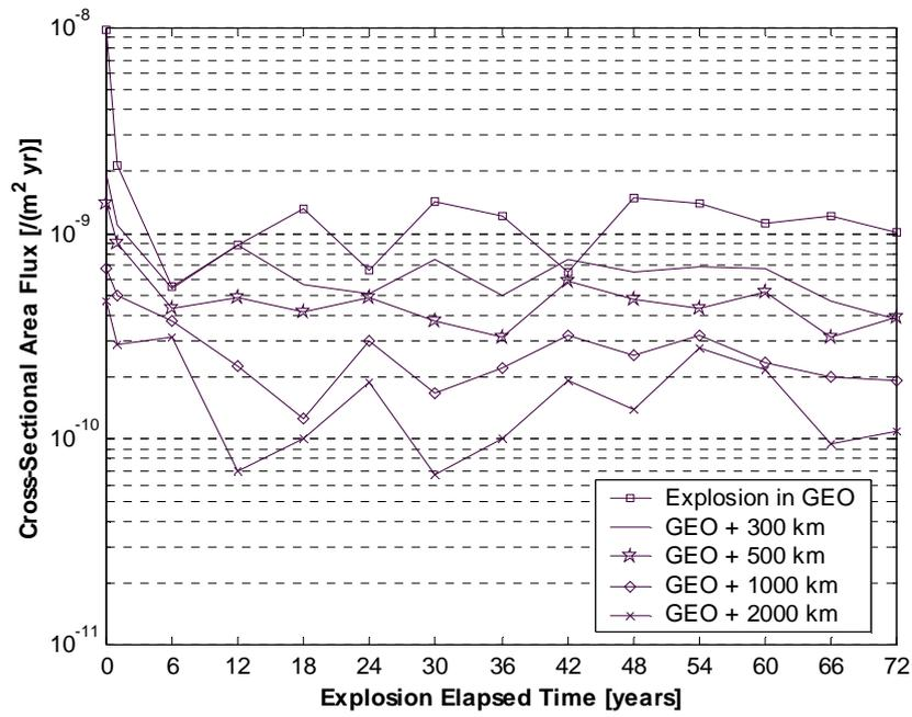
Figure 15. Flux of explosion fragments  $\geq 10$  cm in geostationary orbit, as a function of the breakup altitude and elapsed time
