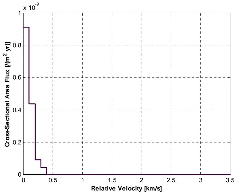
Figure 12. Flux of debris  $\geq 10$  cm in geostationary orbit, as a function of relative velocity, due to an explosion in GEO (explosion elapsed time = 54 years)
