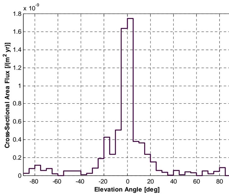
Figure 2. Background flux in GEO, as a function of elevation, of debris  $\geq 10$  cm
