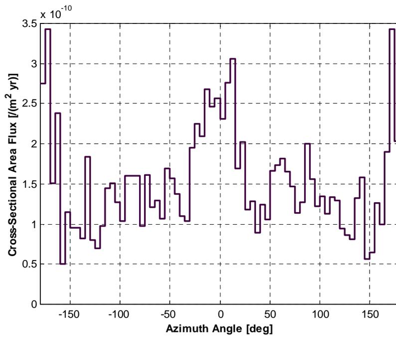
Figure 4. Flux of debris  $\geq 10$  cm in geostationary orbit, as a function of azimuth, due to an explosion in GEO (explosion elapsed time = 0 years)
