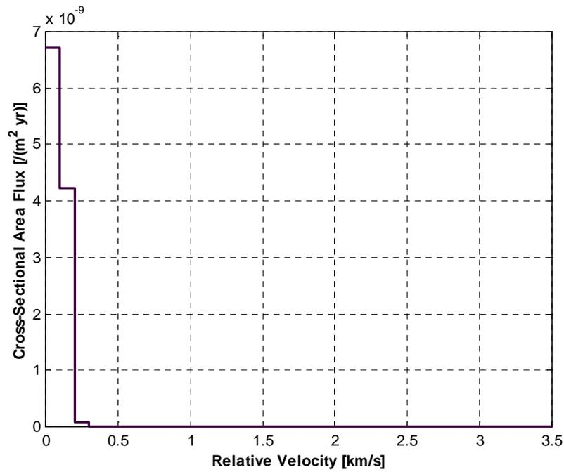
Figure 6. Flux of debris  $\geq 10$  cm in geostationary orbit, as a function of relative velocity, due to an explosion in GEO (explosion elapsed time = 0 years)
