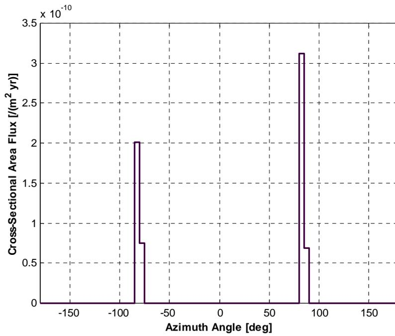
Figure 7. Flux of debris  $\geq 10$  cm in geostationary orbit, as a function of azimuth, due to an explosion in GEO (explosion elapsed time = 24 years)
