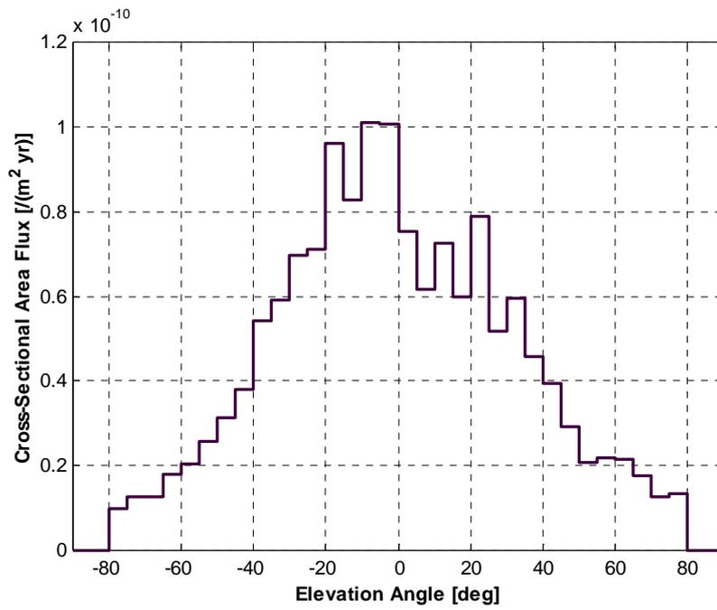
Figure 11. Flux of debris  $\geq 10$  cm in geostationary orbit, as a function of elevation, due to an explosion in GEO (explosion elapsed time = 54 years)
